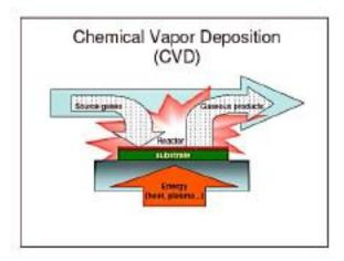
Frequently, volatile by-products are also produced, which are removed by gas flow through the reaction chamber
